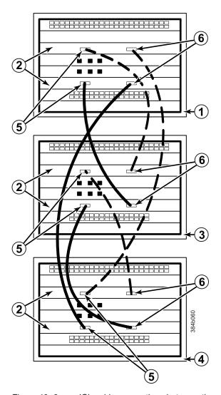
Figure 49. 3-way ICL cable connections between three SAN384B chassis.
